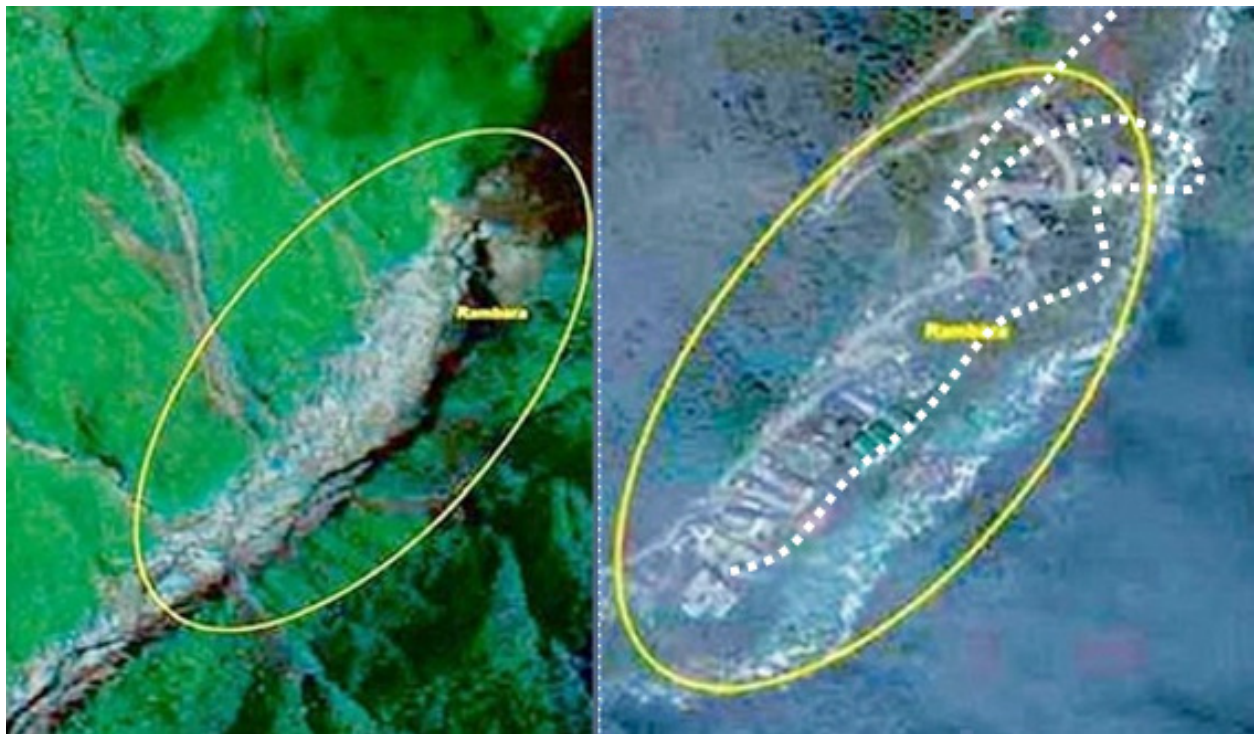
Fig. 7. Rambara area after disaster & before disaster, where road is shown in dotted line. (Resourcesat Image).
