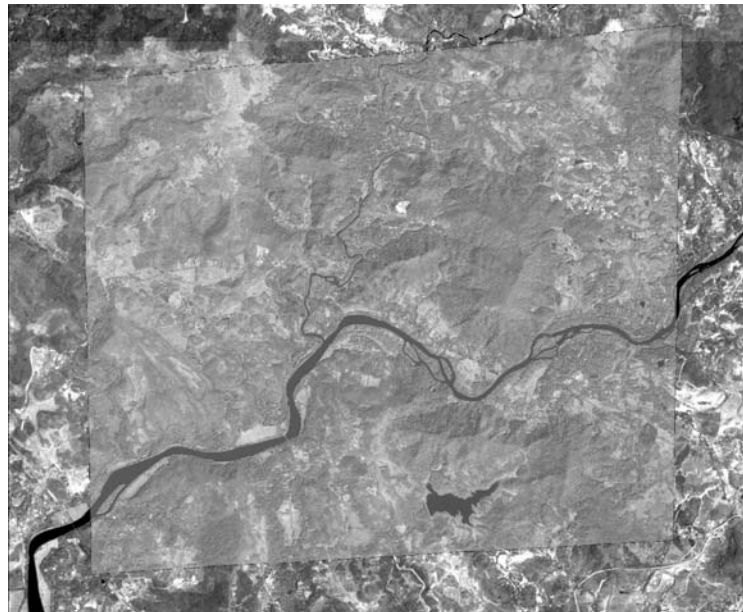
Fig. 5. Cartosat-2 orthoimage overlaid onto mosaiced CartoDEM orthotiles
